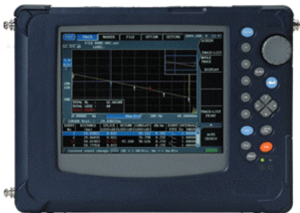
Fig. 6 Example of OTDR for field use
