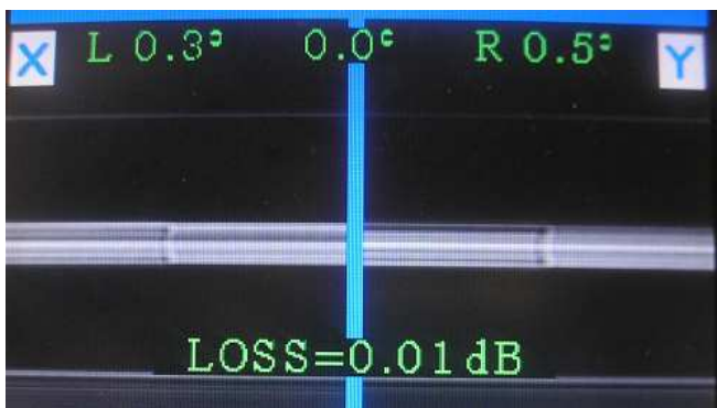
Fig. 2 Splicer screen showing fibers from different manufacturing process
