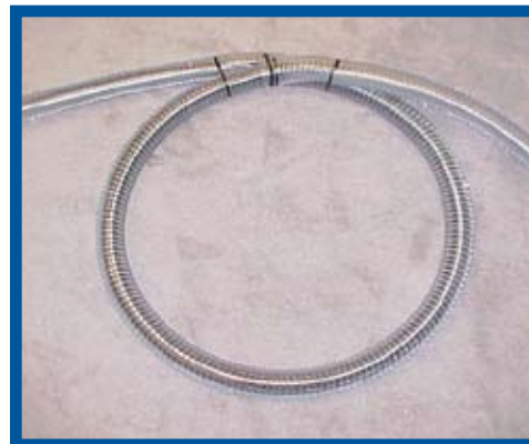
Figure 3: Cable Coil Placed Inside Slit Tube
