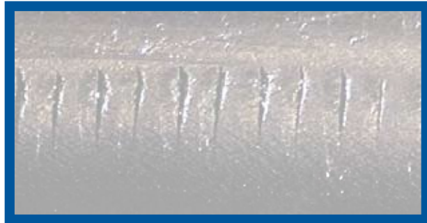
GOOD MARKS Light parallel lines indicate side of rollers are contacting cable
